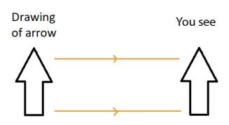
If we hold the paper behind a glass of water the arrow looks like it is pointing in the opposite direction. This is because the light gets bent, its refracted, when it travels through water. When the light rays leave the glass they cross over each other. Light that was on the left is on the light, so the arrow appears to reverse itself!
